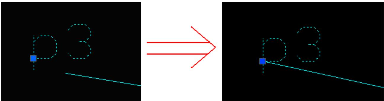
NOTE: When use "straight" to connect "round" and "port number (single text)," need to open the automatic capture AUTOCAD, this can easily capture the center and the text insertion point.
