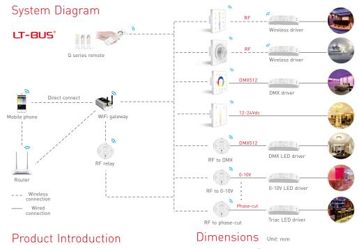
${\bf Q}$  series remote control is a 4 zones control in color circle dimming and slider touch dimming. Color and brightness is displayed by color indicators. Connect to any wireless driver within effective distance and keep the effect in sync. Working with F4-5A, F4-DMX-5A, F5-DMX-4A and touch panel, etc.
