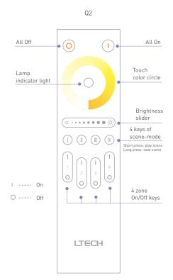
On/Off Mode (8) Short press: switch mode Long press: adjust speed Touch Lamps color circle indicator light Brightness slider ÷ · · · · · · · · · · · White light key 3 keys of scene-mode Short press: play scene Long press: save scene 4 zone O ---- Off On/Off keys LTECH
