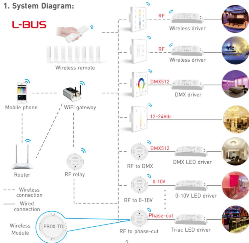
EBOX-TD wireless module applies L-BUS wireless communication protocol and converts it into trailing edge dimming signal through RF wireless communication technology, which is used together with LTECH Triac LED driver and compatible with all Triac series products in the market. Rely on L-BUS wireless technology application, it has removed the complex cabling procedure and expensive technical commissioning fee, to make it more easier for new or retrofit installations.
