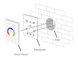
3. screw the baseplate and the back box in the wall firmly.
