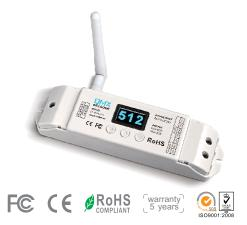
LT-874-5A 4CH CV DMX decoder with OLED display, receiving standard DMX512 protocol data wirelessly. use with our LT-870 wireless emitter, supporting point to point, point to multi-point communication. One emitter can match multiple receivers if using the same frequency, self-testing function also available.
