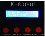
NOTE: The number 4 shows on CHIP position means UCS512 coding mode; 5 means WS2821 coding mode; 6 means SM512 coding mode.
