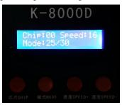
NOTE: When the chip is 00-03, press MODE button for eight seconds can direct write address to UCS512, the interval is three channels.
