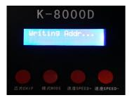
4. After coding, power the light again, press "CHIP" and change to 0, it would be international standard DMX512(1990) agreement play mode. At this time press MODE and SPEED button can switch play mode and adjust speed respectively, like below:
