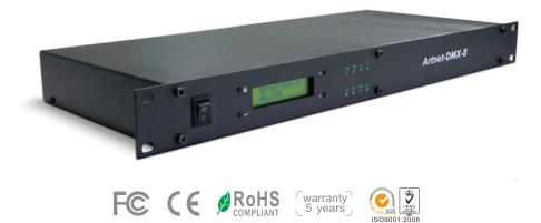
Artnet-DMX converter is the Ethernet Control System based on the Artnet protocol, used to convert the Artnet network data package into DMX512 data, adopting high-speed ARM processor, stable and reliable working. Following Artnet standard protocol, it supports RJ45 network interface and standard DMX512 output interface.
